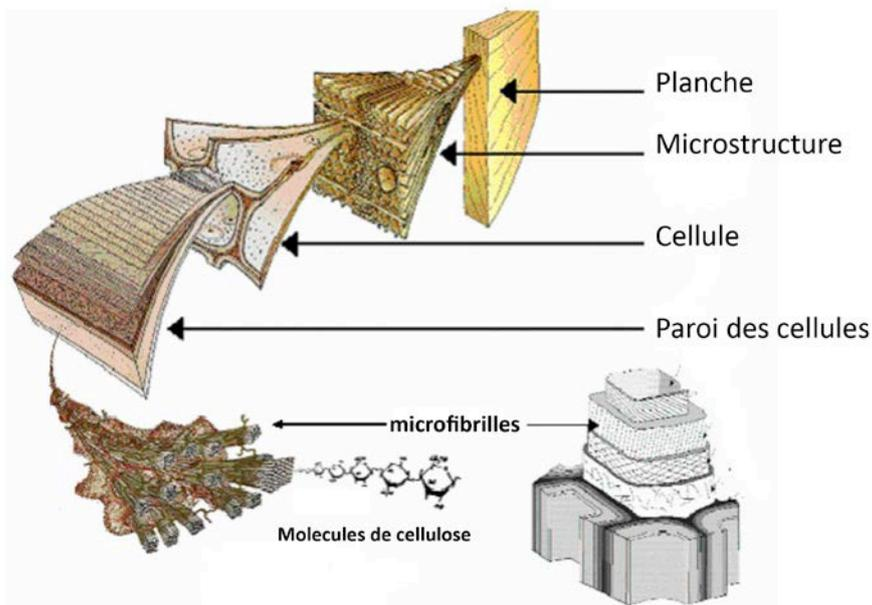
Fig. 7: Structure of wood, showing the cells and microfibrils.
