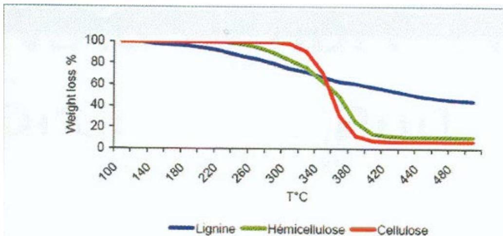
Fig. 8: TGA thermograms (weight loss) of plant fibre components
