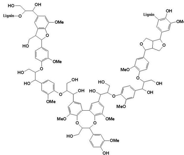
Fig. 4: chemical structure of lignin.
