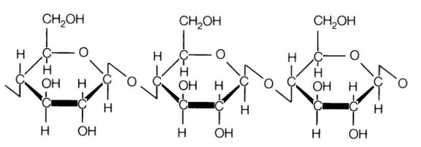
Fig. 2: chemical structure of cellulose.
